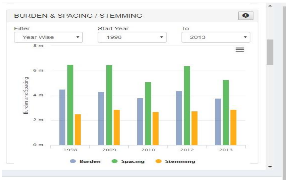
Figure 6 - Burden and spacing/stemming
