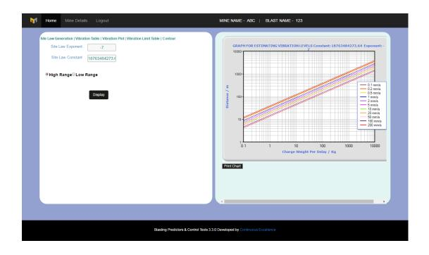
On click of Display button, the results will be displayed in the graph format, in which x-axis define the Charge Weight per Delay (in kg) and y axis will shows the Distance (in meters). The user can use the default parameters and edit these parameters as per their operational requirement. User can select either high range or low range.
