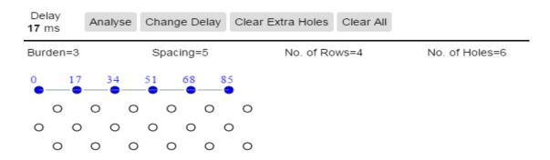
4. Repeat the process 1 - 3 to connect the holes to be tied.
