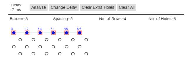
3. After that click on last selected hole. User gets tie lines between all holes and holes filled with blue colour with without red square and delay will appear above the holes.
