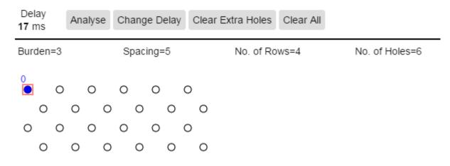
2. Move the mouse cursor to next hole which is to be connected from active hole. On click selected hole blue colour tie lines will appear between all holes those come in line of selected two holes. All holes also activated with red colour square outside and filled with blue colour.
