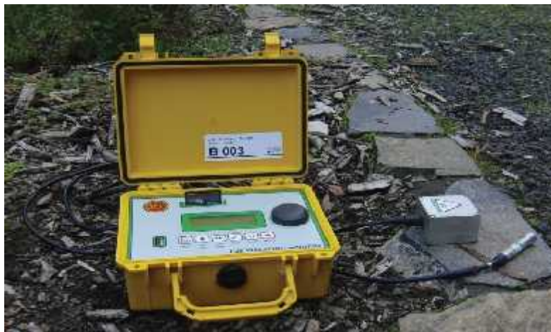
Figure 2 Continuous Monitoring Blast Vibration meter with GPS included
